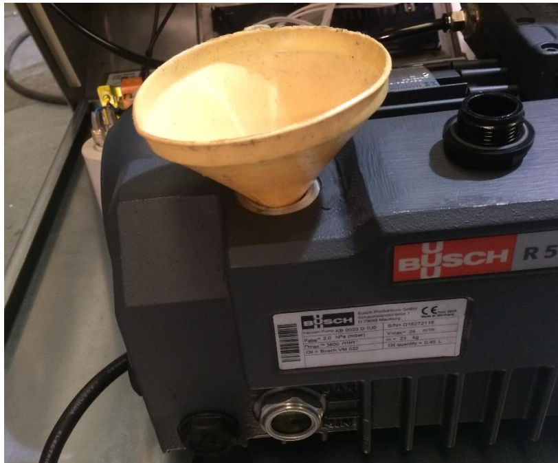
Illustration 6. Remove the oil filling plug and refill with new oil
