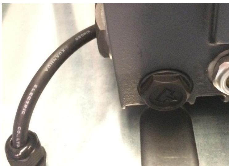
Illustration 4. Remove the oil drainage plug
